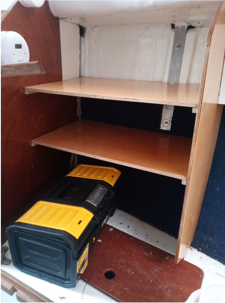
Larger cupboard and new insulation installed after painting
